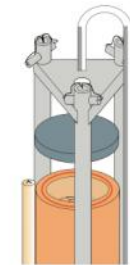
Fig. 6. Setup 6: permeability measurements for use with GC or MS.
