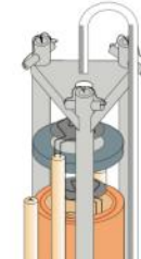
Fig. 3. Setup 3: transport number measurements by EMF of concentration cell or fuel cell testing with seal, H2N# and INH2N# electrode contacts.
