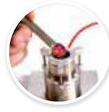
The Small-Volume Test Kit was originally developed with the US Navy specifically for testing energetic materials. The effectiveness of the accessory in reducing the volume requirements for testing samples make it ideal for characterizing the thermal conductivity of liquid samples. The SVTK is commonly applied in testing nano and heat transfer fluids, as well as emulsions.
